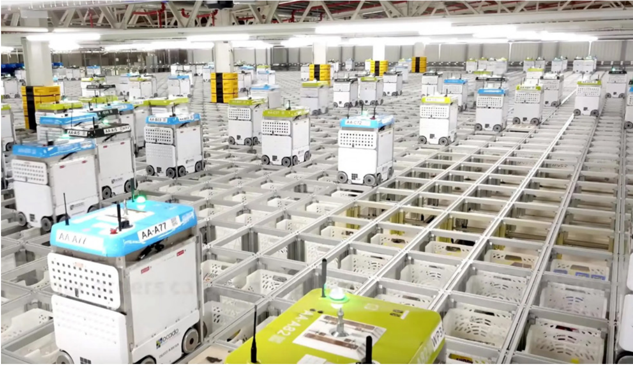
Ocado Group's cube storage system for e-grocery fulfillment
